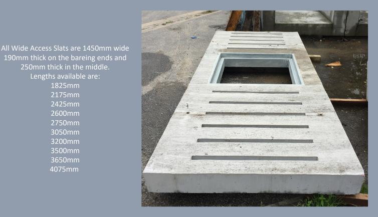
190mm thick on the bareing ends and 250mm thick in the middle. Lengths available are: 1825mm 2175mm 2425mm 2600mm 2750mm 3050mm 3200mm 3500mm 3650mm 4075mm
